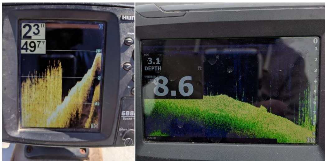
Image 1. Down-imaging SONAR images showing edge of milfoil coverage and the height of milfoil plants.
